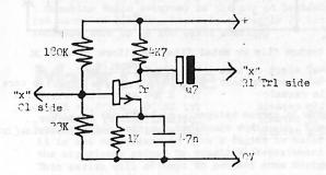
With reference to Fig.1, break the connection at Cl,Rl,Trl,and insert this circuit for pre-emphasis. I'l is BC549,BC109 etc.
